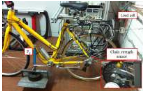
Figure 8. Experimental setup for the estimation of the torque acting on the pedal starting from the chain strength sensor.
