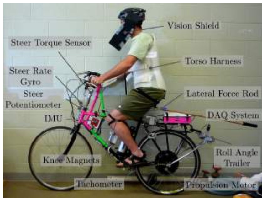
Figure 5. The instrumented electric bicycle. The rear wheel hub contains the electric motor and both the battery and motor controller are mounted mid-frame.
