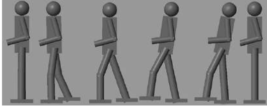
Figure 9: A single step of the biped robot. The robot moves from right to left as the time passes.
