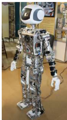
Figure 1: Testing anthropomorphic robot AR-601M, the shell is removed.
