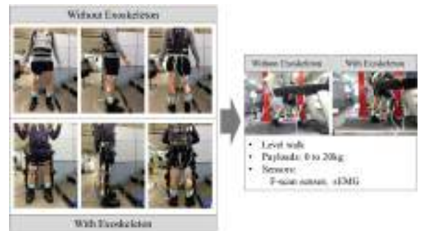
Fig. 6: Experimental setup of the power augmentation effect in level walking.
