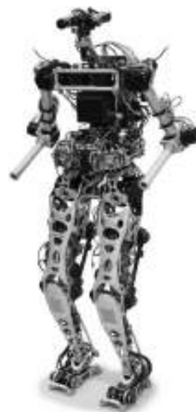
Fig. 1. Photograph of the 25-DOF humanoid walking robot LOLA .
