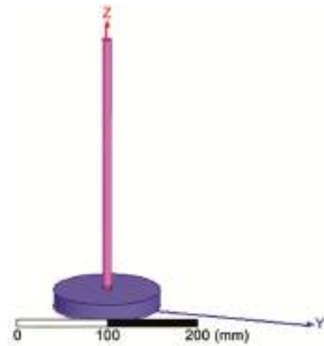
Fig. 4 — Plasma Antenna model of 0.5 cm radius and 30 cm length.
