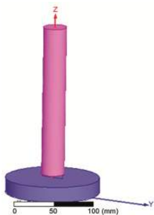
Fig. 5 — Plasma Antenna model of 1.5 cm radius and 20 cm length.
