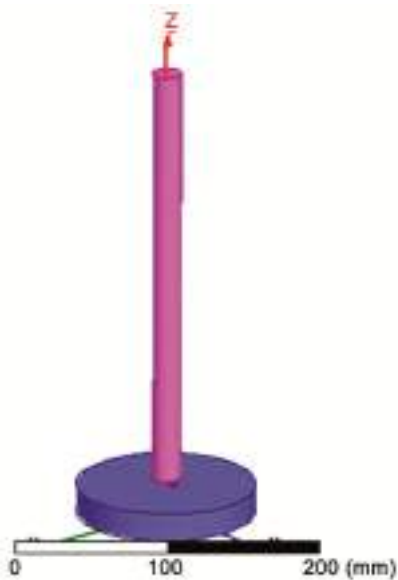
Fig. 3 — Plasma Antenna model of 1.0 cm radius and 30 cm length. 1.5 cm but different lengths of 20 cm and 10 cm shown in Fig. 5 and Fig. 6, respectively.
