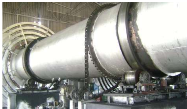
Fig.1. Rotary kiln arrangement
