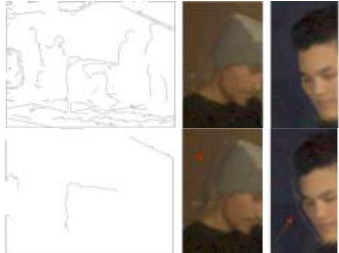
Fig. 5 A large Canny threshold may imply corona-like effects (lower), whereas a more sensitive edge detection avoids those (upper).
