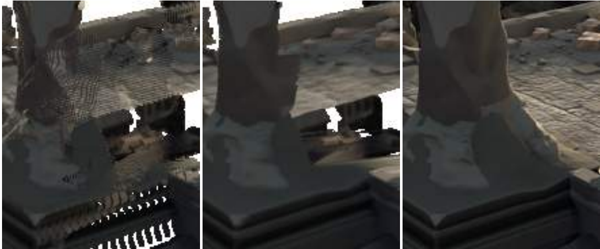
Figure 6: Artifacts due to missing connectivity (detail from the temple2 sequence): CPU version (left) with background objects shining through foreground; OpenGL version (middle): no artifacts, the partly missing foreground objects are due to occlusion in the input frame; ground-truth image (right) This is a particular difficult projection, where the camera was rotated by nearly 90 degrees between input and output frame
