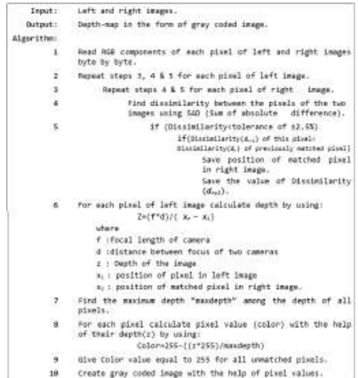
Fig. 2. Proposed algorithm for depth-map creation
