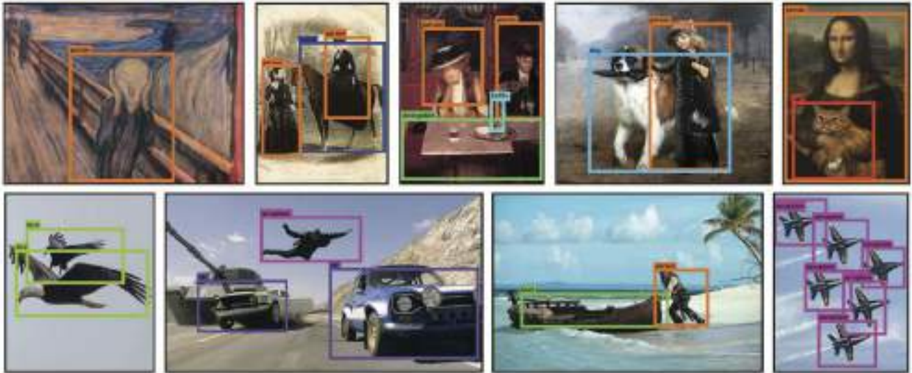
Figure 6: Qualitative Results. YOLO running on sample artwork and natural images from the internet. It is mostly accurate although it does think one person is an airplane.
