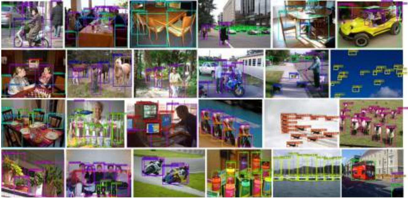
Figure 4: Qualitative results of RefineDet512 on the PASCAL VOC 2012 test set (corresponding to 85.0% mAP). VGG-16 is used as the backbone network. The training data is 07++12+COCO.
