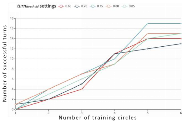
Fig. 4. The performance of our simulator when considering different number of training circles and different value of turn_{threshold} settings.
