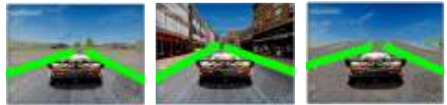
Fig. 6. Draw out the lanes by using Hough Transfer algorithm.
