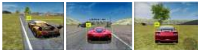
Fig. 7. Obstacle detection for the car by implementing YOLO in our simulator.
