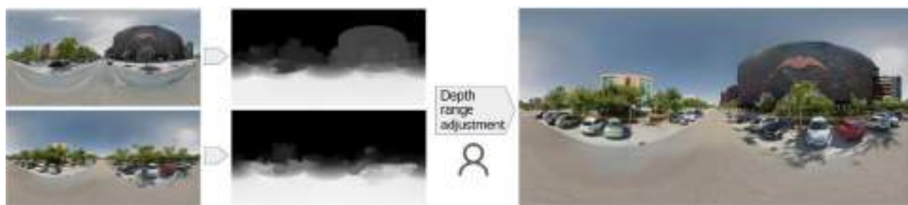
Fig. 1 Spherical panorama compositing through depth estimation. We first obtain the relative depth maps for the source panoramas and then, the user interactively modifies depth ranges to obtain the desired composition, shown at the right (Source of panoramas: Street View [17])
