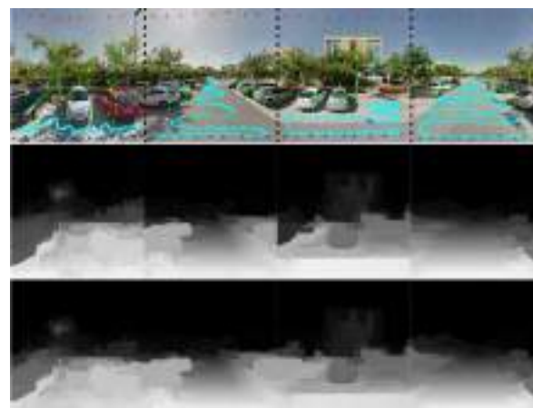
Fig. 6 Depth maps for the left, front, right and back faces of a cube map: Provided input (top), using DfSI separately (center) and using our method (bottom). There are depth discontinuities in boundaries when DfSI is applied separately
