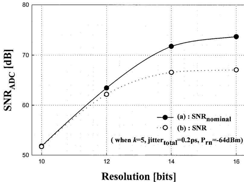
Fig. 8. Relationship between SNR<sub>ADC</sub> and resolution bits.
