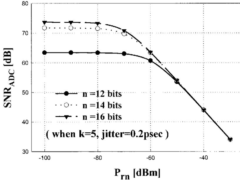
Fig. 6.  $SNR_{ADC}$  versus ADC input-referred receiver noise power ( $P_{rn}$ ).
