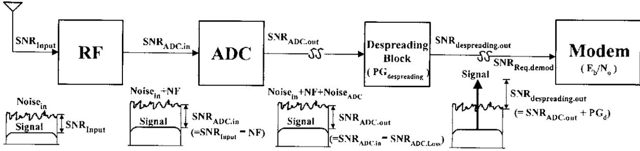
Fig. 12. Cascaded SNR of desired signal.
