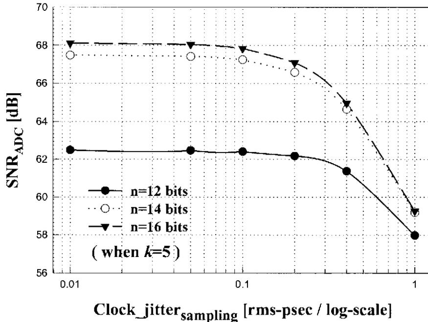
Fig. 9. Relationship between SNR<sub>ADC</sub> and clock jitter.
