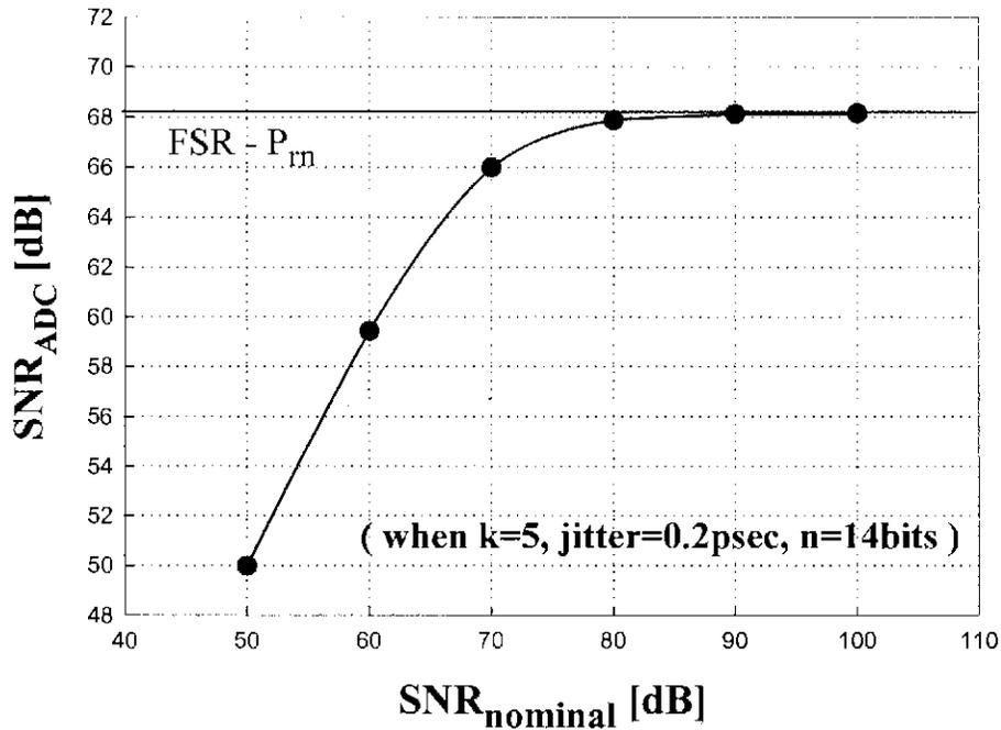
Fig. 7. SNR<sub>ADC</sub> versus SNR.
