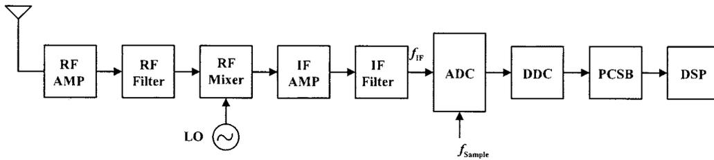
Fig. 3. Basic architecture of Digital-IF Transceiver.
