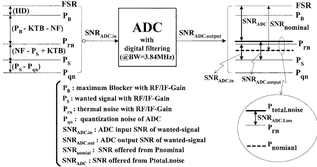
Fig. 5. Signal levels of ADC input/output.
