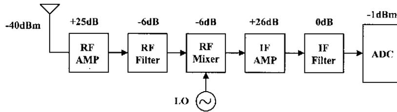
Fig. 16. RF/IF section of digital-IF receiver.
