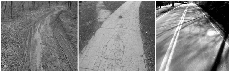
Figure 12: Video images taken on three of the road types ALVINN modules have been trained to handle. They are, from left to right, a single-lane dirt access road, a single-lane paved bicycle path, and a lined two-lane highway.
