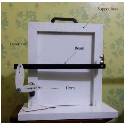
Figure 3. Main parts of the system
