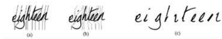
Figure 2. Segmentation using Shortest Path of a Graph of Gray Level Image (a) Segmentation Intervals (b) Segmentation Paths (c) Segments [11]
