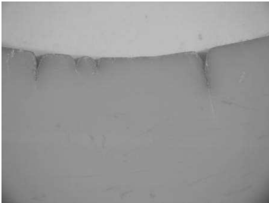
Figure 8. The cross section of the pipe wall after reaction with SO 2 to visualise the hydroperoxides.
